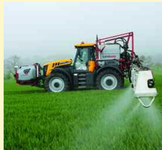
The aluminium boom on the Landquip sprayer means the move to 36m has come without a big weight penalty.
