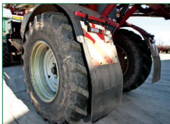
... and also made these mudguard extensions for the sprayer's rear axle.
