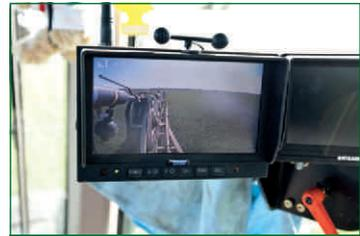
Cameras around the sprayer add an extra dimension to spraying visibility.
