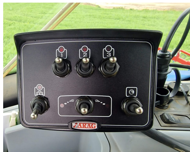
3 section electric switch box for individual left & right hand row switching and rear centre spray bar Electric master & pressure regulation
