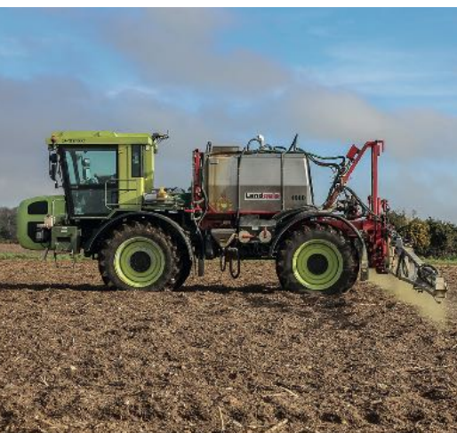
Even weight distribution helps reduce compaction and deep wheelings and the proven Landquip Contractor heavy-duty aluminium booms travel well and are ruggedly built.
