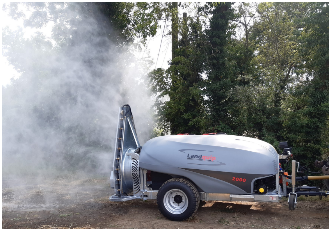
800mm reverse / forward intake fan 8 nozzles + 1 directionally adjustable nozzle
