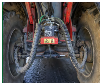
The PTO-driven hydraulic pump supplies up to 130hp to drive the sprayer's wheels.
