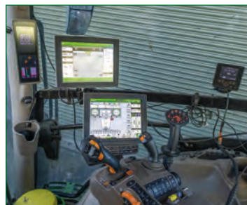
An Arag terminal with extended terminal looks after sprayer control and monitoring.
