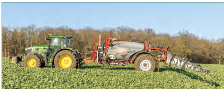
The PowerTrac's driven axle has created a six-wheel drive combination, boosting traction for a wide variety of field conditions, and greatly improving the timeliness of applications.
