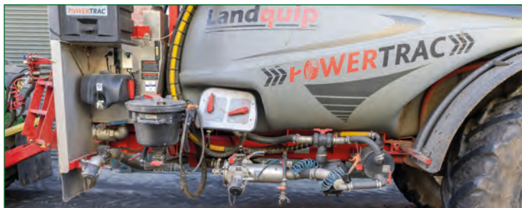
The straightforward filling area is configured with 3in pipework. The sprayer pump that is driven hydraulically from the tractor, can fill the tank in about seven-to-eight minutes.
